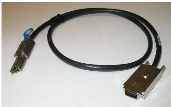
Figure E-16: The CBL-0166L Cable
