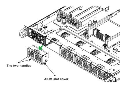
Note: This AIOM module does not support hot plug. Please turn off the AC power and remove the power cord from the wall socket before installing or removing an AIOM module.
