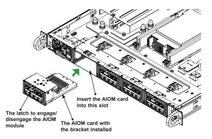
Note: A computer system should not be operating with an empty AIOM slot. All slots should be populated with AIOM modules, AIOM slot covers, or combinations of both.
