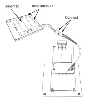
10. Mount the installation kit into a 2.5 inch hard disk drive bay. Insert the drive bay back into the system. Reinstall the system cover, reattach the power cord and power on the system.
