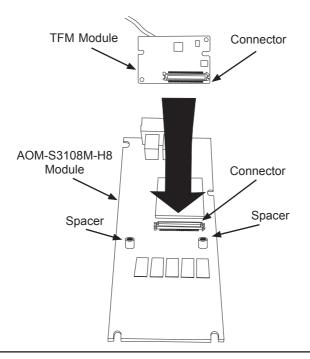
Press the TFM module down firmly to seat the module correctly in the slot. Insert two screws provided in the spacer kit and tighten them to secure the TFM module.
