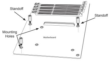
**Note**: Module graphics in this manual are based on the latest revision. Your module and motherboard may or may not look exactly the same as the graphics shown.  Before installing the AOM-S3108-H8 module onto the motherboard, install the spacers onto the middle set of holes on the module. Secure the spacers by tightening the screws on the bottomside of the module.
