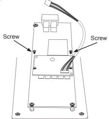
With the TFM module seated in the AOM-S3108-H8 module, place the Supercap battery in the installation kit. Connect the Supercap wire with the TFM module wire.
