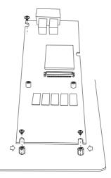
Align the connector on the bottom of TFM module with the connector on the AOM-S3108M-H8 module.
