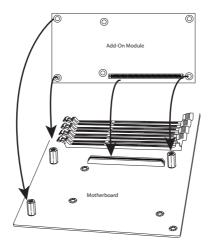
6. With the add-on module securely seated in the slot, insert Pan Head #6 screws into the standoff holes and tighten them with a Phillips screwdriver.
