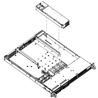
Figure 5-13: Removing the Power Supply
