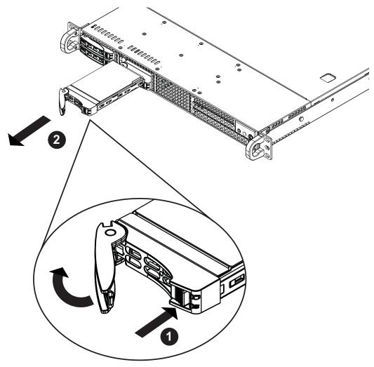
Figure 5-2: Removing Hard Drive
