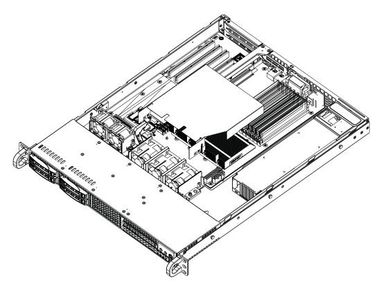
Figure 5-10: Air Shroud Installation
