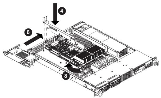
Figure 5-9: Chassis with a Riser Card
