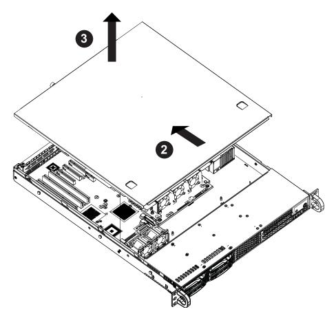
Figure 5-1: Removing the Chassis Cover
