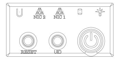
Figure 4-1. Control Panel Buttons and LEDs
