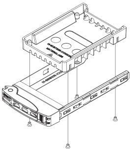
Figure 5-3: Hard Drive Carrier
