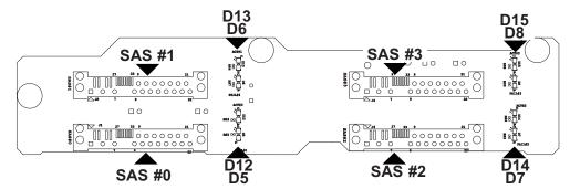
Figure C-4: Rear Connectors and LEDs
