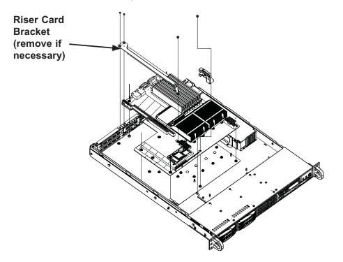
Figure 5-7: Installing the Motherboard
