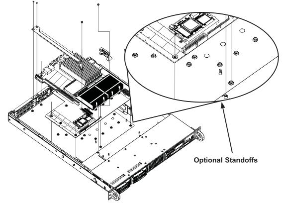
5-6 Installing the Motherboard
