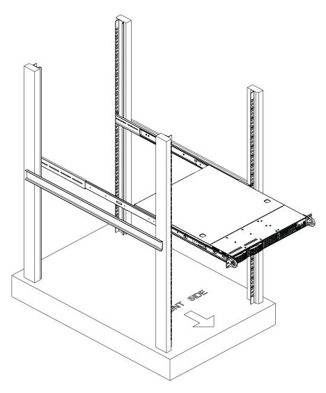
Figure 6-4: Installing the Chassis
