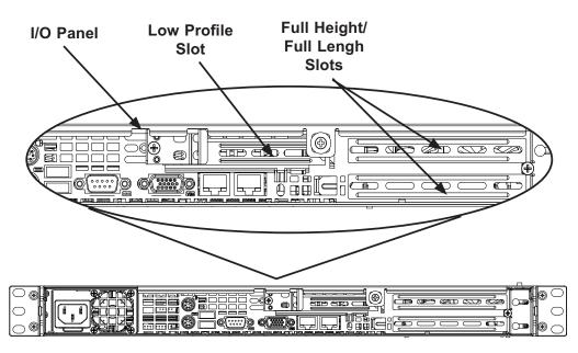
Figure 5-8: SC111 Rear - Full Height/Full Length Slots and Low Profile Slot
