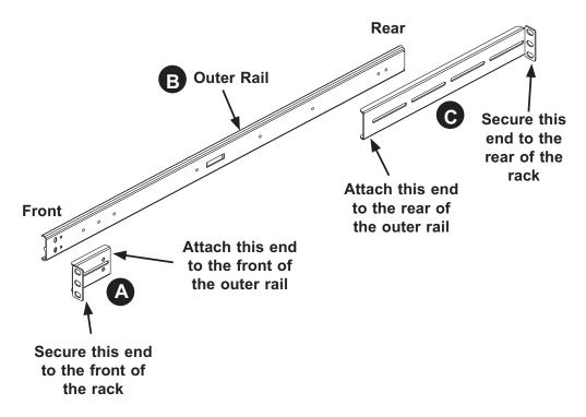
Figure 6-3: Assembling the Standard Outer Rails
