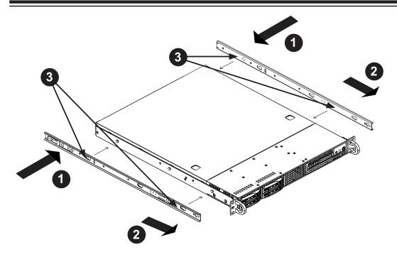
Figure 6-2: Installing the Inner Rails
