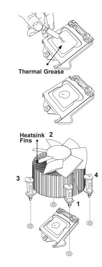
Recommended Supermicro heatsink: SNK-P0046A4 or SNK-P0051AP4 active heatsink (2U+ or 4U chassis)
