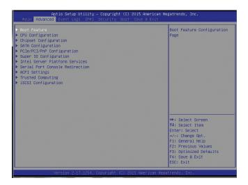
**Warning**: Take caution when changing the Advanced settings. An incorrect value, an inaccurate DRAM frequency, or a wrong DRAM timing setting may make the system unstable. When this occurs, revert the setting to the manufacture default settings.
