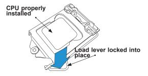
**Note:** You can only install the CPU inside the socket in one direction. Make sure that it is properly inserted into the CPU socket before closing the load plate. If it doesn't close properly, do not force it as it may damage your CPU. Instead, open the load plate again and double-check that the CPU is aligned properly.
