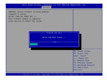
5. After the BIOS recovery process is complete, press any key to reboot the system.
